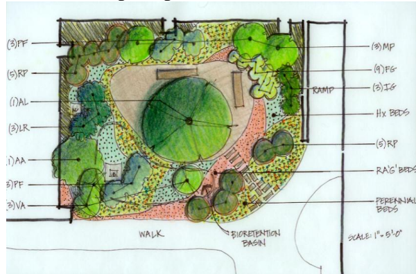
Figure 2: Example of Concept Design for Rain Garden eligible for inclusion in required open space
